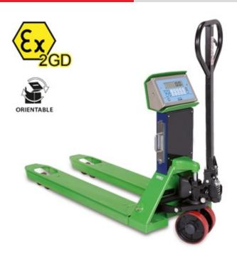
ATEX pallet truck scale for use in hazardous areas (ZONES 1 & 21 & 2 & 22) with Ex II 2G IIB T4 Gb X and Ex II 2D IIIC T197°C Db X protection. Also available in a version approved for legalfor-trade use. Manufactured, calibrated and adjusted in Italy by Dini Argeo, using certified sample weights.
